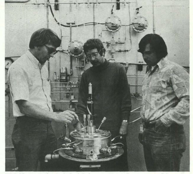
THREE of the many Sandians involved in the high temperature test cells project. Here, cell designer Leon Seibel (8312) explains the working end of the high pressure cell to project engineer Larry Weirick (also 8312) and Pete Roybal (8314), who designed the facility in which the cell sits, including the complex plumbing system.
